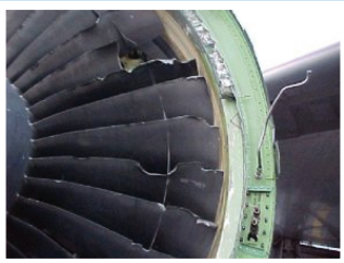
Bird damage to plane engine, Jan. 2001 Photo Credit: Federal Aviation Association
