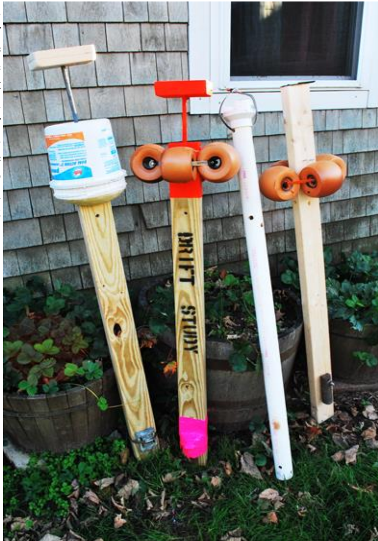
Figure 1. Variations in the "mast" of the surface drifters with Eddie 1.2, Eddie 1.1, Rachel 1.1, and Eddie 1.0 (left to right).
