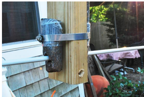
Figure 2b. Another option for securing ballast: run spars through holes in window weights.
