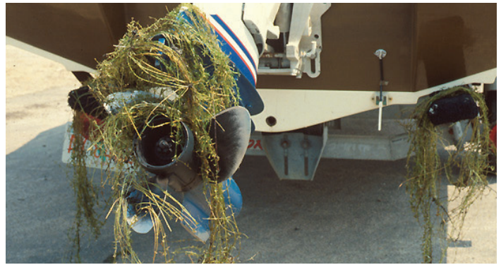
Hydrilla clogging a boat propeller. Credit Jeff Schardt, University of Florida.
